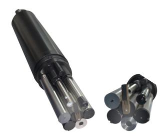
BOQU Online Multi-Parameter Water Quality Sensor is suitable for long-term field on-line monitoring. It can achieve the function of data reading, data storage and real-time online measurement of temperature, water depth, pH, conductivity, salinity, TDS, turbidity, DO, chlorophyll and blue-green algae at the same time. it also can be customized according to special requirements.
